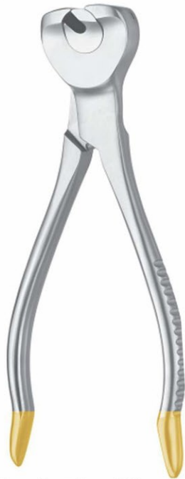
Wire Cutting Plier (TC) For Soft Wires Up to 3.5 mm Ø, For Hard Wires Up to 2.5 mm Ø 16 cm TS-10-165
